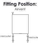
All Dimension are in mm Max.Working Pressure = 10 Bar Max.Working Temprature=95° C Inlet / Outlet : 1/2" BSP
