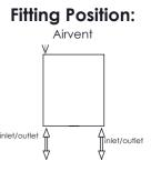
All Dimension are in mm Max.Working Pressure = 10 Bar Max.Working Temprature=95° C Inlet / Outlet : 1/2" BSP
