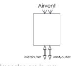
All Dimension are in mm Max.Working Pressure = 10 Bar Max.Working Temprature=95° C Inlet / Outlet : 1/2" BSP
