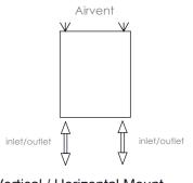
Vertical / Horizontal Mount All Dimensions are in mm Max.Working Pressure: 8 Bar Max.Working Temperature: 95° C Inlet / Outlet : 1/2" BSP Fuel : E/H/D
