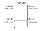
All Dimension are in mm Max.Working Pressure = 10 Bar Max.Working Temprature=95° C Inlet / Outlet : 1/2" BSP
