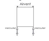
All Dimension are in mm Max.Working Pressure = 10 Bar Max.Working Temprature=95° C Inlet / Outlet : 1/2" BSP
